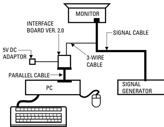
Figure 4-1. Setup 1, With Signal Generator
